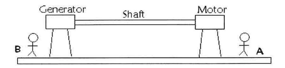
Figure 26. The motor turns the generator using a shaft.
