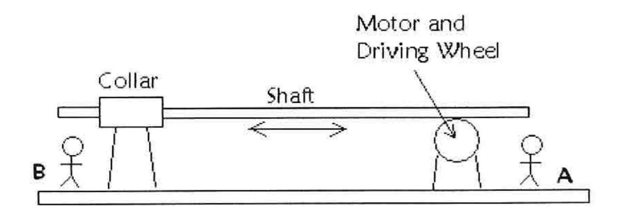
Figure 27. A motor moves a shaft linearly through a collar.
