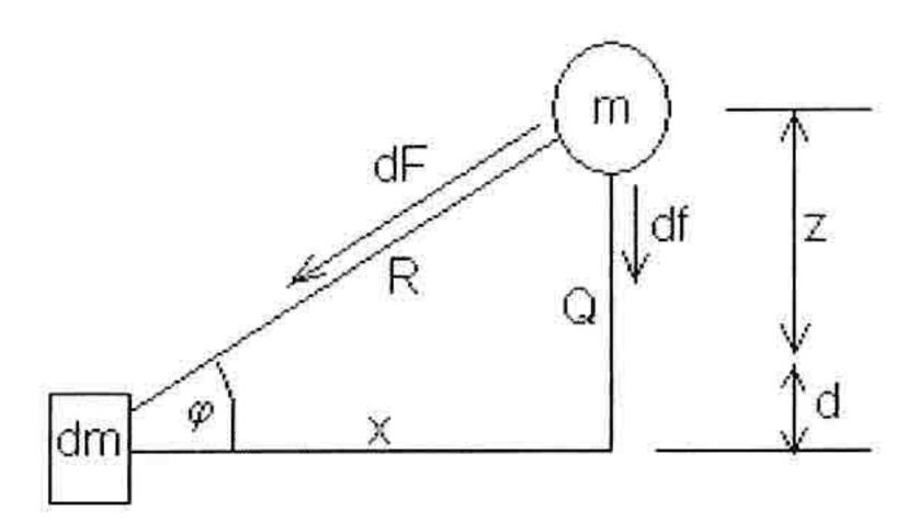
Figure 2. Q-x plane view of the forces.
