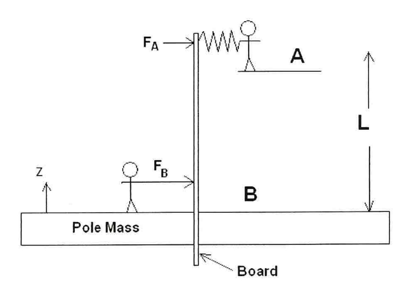
Figure 3. Horizontal force experiment.
